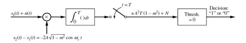
Figure 7-14 Correlator realization of optimum receiver for PSK.
